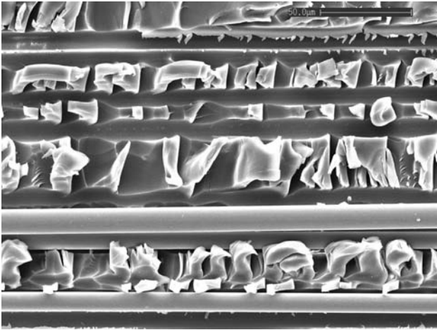
Fig. 2 Fracture surface micrograph from an interlaminar short beam shear sample
